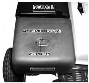
The Air Cleaner Cover (51) is held in place by a Wing Nut (47). Remove it. (See Figure L.)
